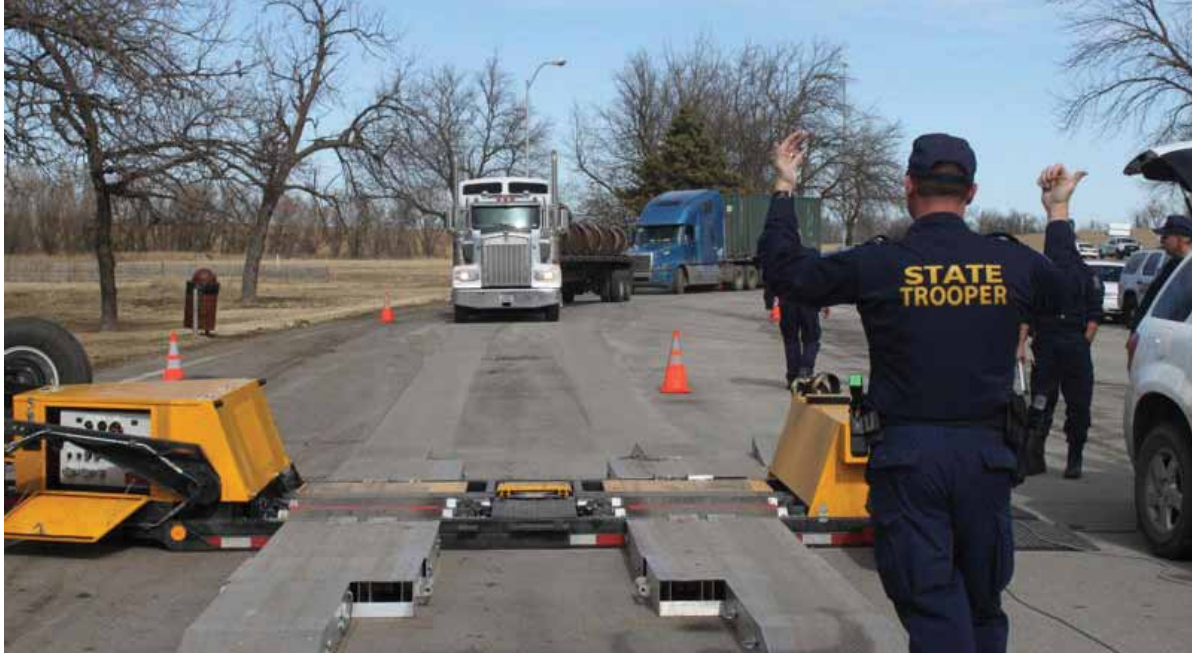
A MCSAP trooper gives a CMV driver hand signals to direct the CMV onto the PBBT.
